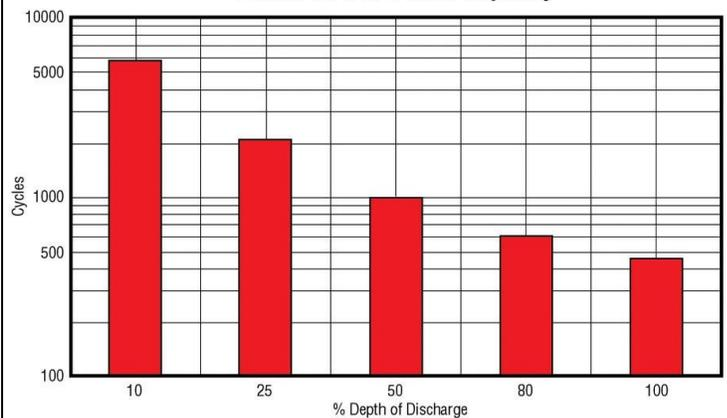
Cycle Chart applies to all MK Gel batteries (except 8GGC2 cycle chart x 2 and 8G31DT cycle chart x .67).
