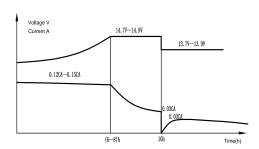
The first stage:at constant current 0,12CA-0,15CA charge,the voltage is up to 14,8V and turns to se
